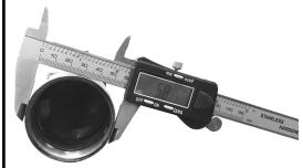
Example. For the scope shown here, the caliper reads 58.21mm. The matching day scope adapter would be 58mm. The part number that needs to be ordered is therefore: DSA-58.
